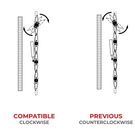
In the case of wall mounting, the above drawingis to be interpreted as the front view of the system (as seen from outside the building). In the case of roof assembly, the above drawing shows top view. The figure shows a view of the closed system on the left. You can choose between feathers that open clockwise or counterclockwise determining the this way determining the opening side of the feathers.
