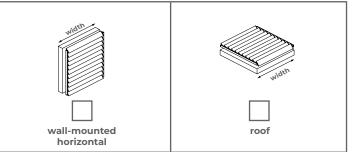
The SUNBREAKER 210 system can be installed in a niche 3or on a substructure. NO BRACKETS FOR FAÇADE MOUNTINC!!!
